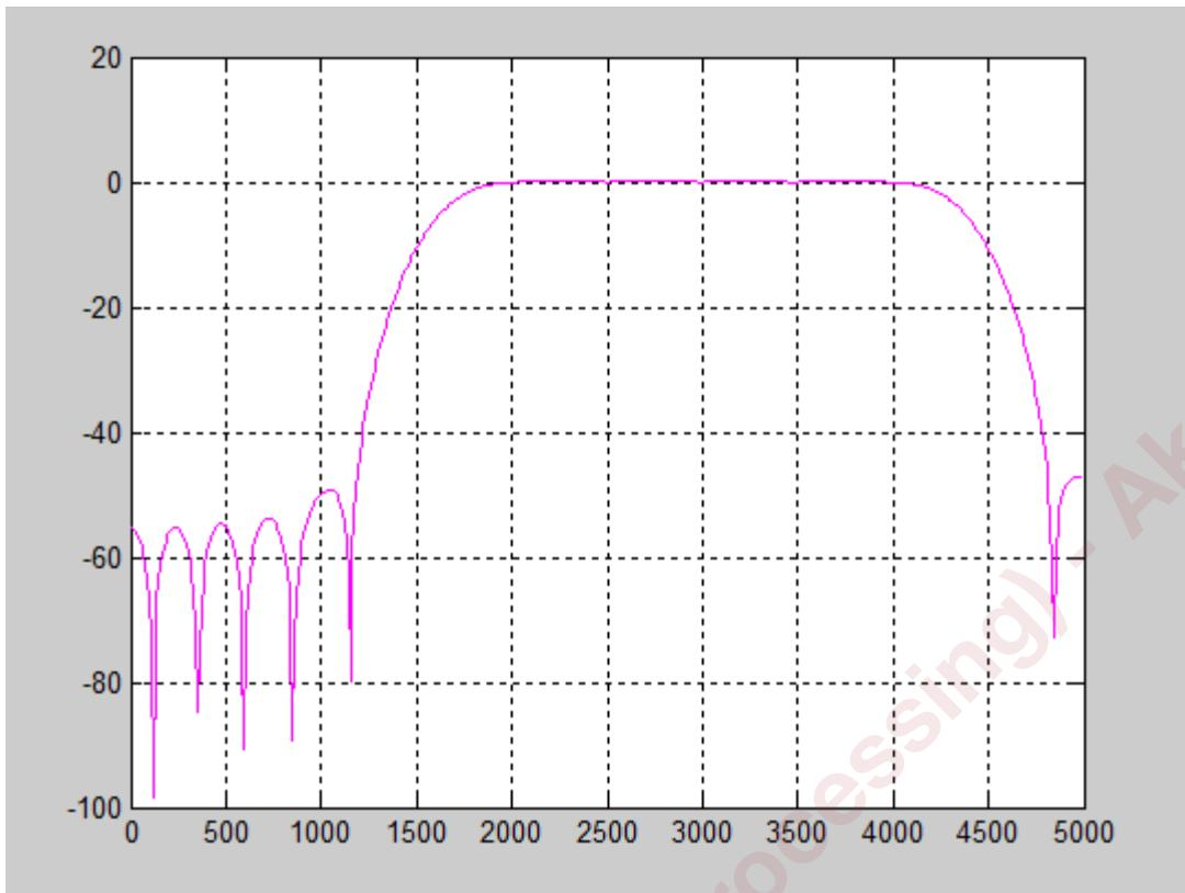
Clearly, it is visible that the pass band is between 2000 to 5000 Hz (nearly)
